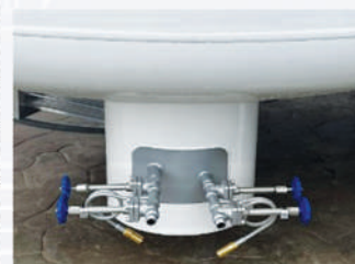
Valve group siphon design with outlet from lower grenade
